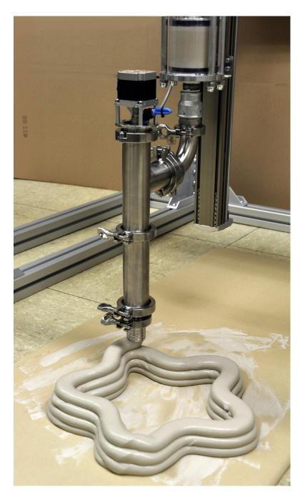
Large-scale mixing print head from stainless steel 304 with stepper motor Nema23 for mortar/concrete.
